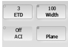
Figure E-3. Example of keys with filled circles indicating visibility in Basic mode.
